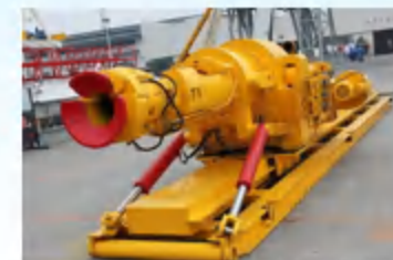
Top Drive Equipment
